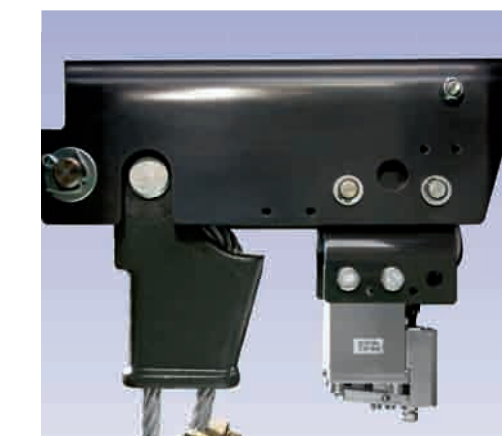
Load registered at rope suspension via spring travel and safety limit switch. Chain hoists have an easy-to-adjust slipping clutch.
