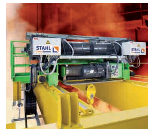
As standard with two synchronously controlled hoists and brakes.
