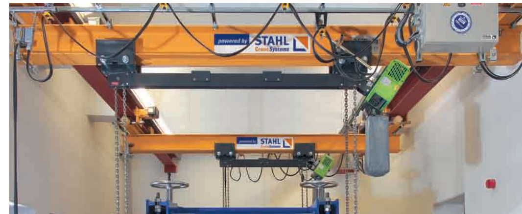
Absolutely synchronous hoisting motion thanks to a single hoist motor, load chains run absolutely in parallel even if load is uneven.
