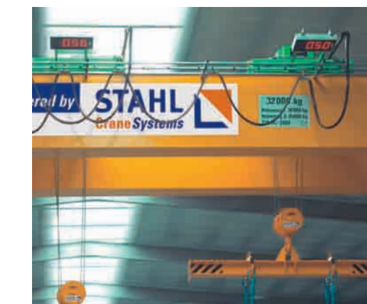
With large-format four-figure load summation for monitoring the total load on both hooks.
